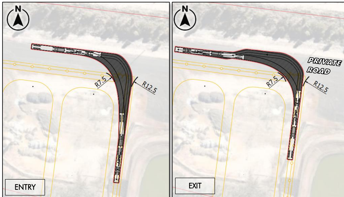
Figure 3.6: TYPE 1 ROAD TRAIN MANOEUVRING – EASTERN-MOST BESS SITE
